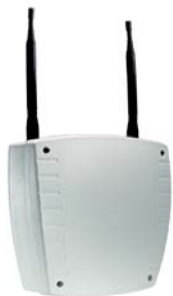
RFP L34 IP with dipole antennas
